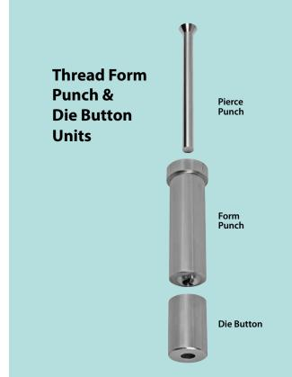
Dayton Thread Form Punch & Die Button Units (available in sets or as individual parts) offer you a single-step, in-die method for punching and forming threads. Dayton Thread Form Units offer many features and benefits over regular hole-tapping systems:
